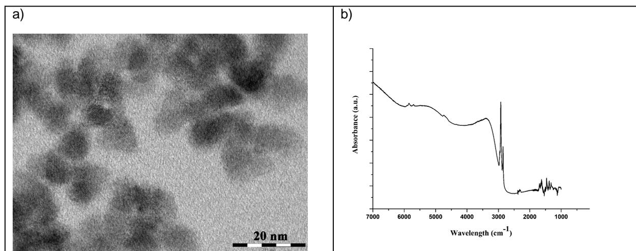
**Fig. 2.** (a) TEM Image of HgTe QDs; (b) Absorption spectra of HgTe QDs.
