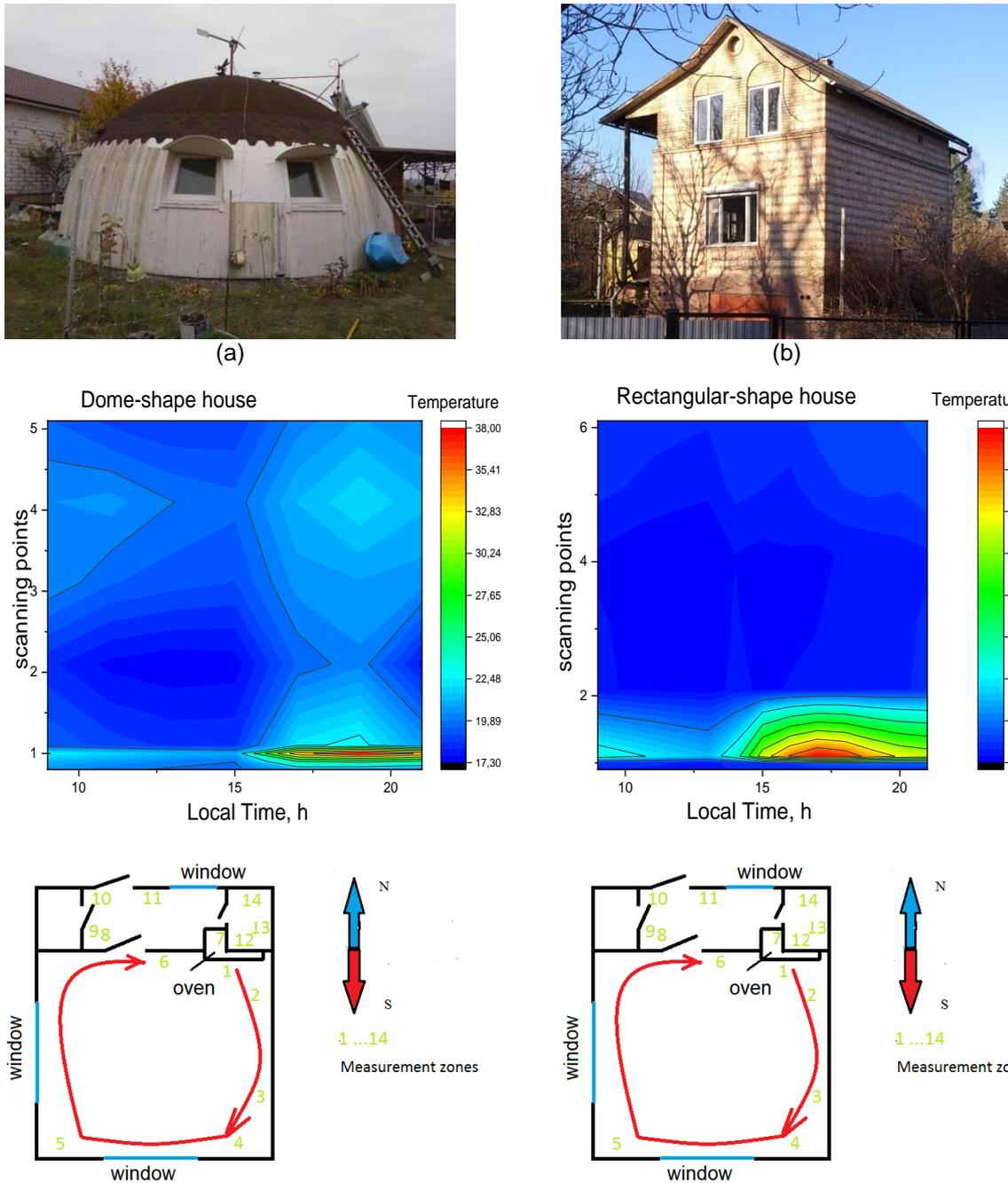
**Fig. 2.** Test buildings (photo on the top), temperature distributions (maps in the middle) for houses of different shapes, and plan of IR sensing (at the bottom, red arrows correspond to the measurement steps), as measured on the same day: (a) dome-shape house, (b) rectangular-shape house.
