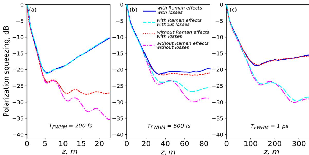
**Fig. 1.** Polarisation squeezing simulated for pulse durations of 200 fs (a), 500 fs (b), and 1 ps (c) using sets of 1000 independent realizations. Here the nonlinear Kerr coefficient is  $0.093$   $(W\ km)^{-1}$ , dispersion is  $-28.0$   $ps^2/km$ , fiber loss is  $1$   $dB/km$ , central wavelength is  $1.5$   $\mu m$ , temperature is  $300$   $K$
