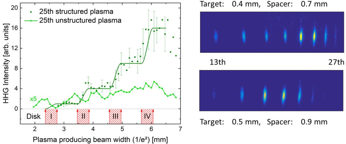
**Fig.2. (a)** Stepwise increase of the intensity of the 25<sup>th</sup> harmonic with the number of plasma jets; **(b)** control of QPM by choosing the target width and spacing.
