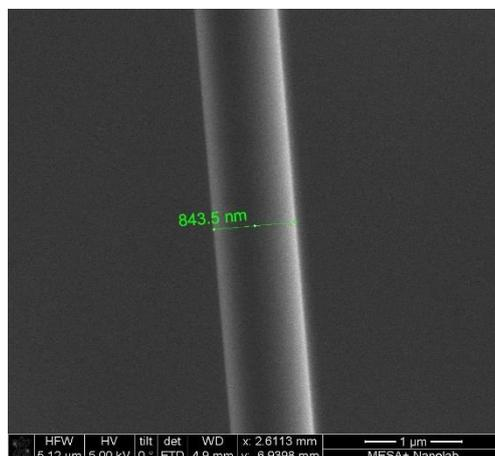
**Fig. 2.** Optical Fibre Taper Diameter in SEM
