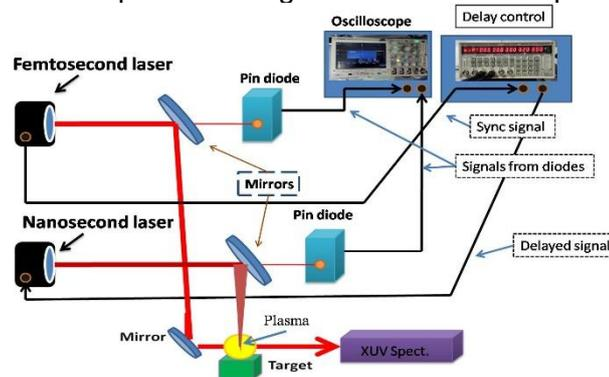
**Fig. 1.** Schematic of the experimental setup for two laser HHG experiments with tuneable delay between heating nanosecond pulse and probing femtosecond pulse
