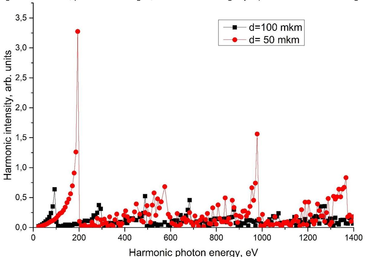
**Fig. 1.** The QPM spectra generated by Argon MGM interacting with two-colour laser field formed by the fundamental and the second harmonics of Ti:Sa laser ( $\lambda=800$  nm). Calculations have been done for pressure 230 mbar and total MGM (25 jets for curve black curve with squares, 50 jets for red curve with circles) length  $L=0.5$  cm
