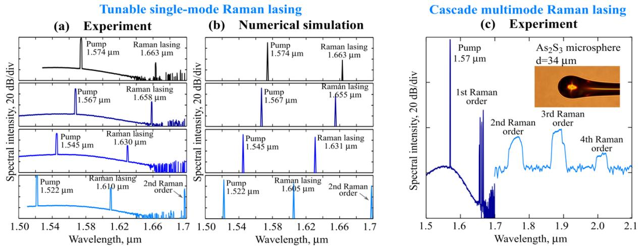
**Fig. 1.** Experimental spectra of tunable single-mode Raman lasing (a) and the corresponding numerically simulated spectra (b) in 34- $\mu\text{m}$   $\text{As}_2\text{S}_3$  glass microsphere [12]. (c) Experimental spectrum of four-cascade Raman lasing recorded by OSA (dark blue curve) and by PbSe detector plus monochromator (light blue curve) [12]. The inset shows the microphoto of the used home-made  $\text{As}_2\text{S}_3$  glass microsphere.
