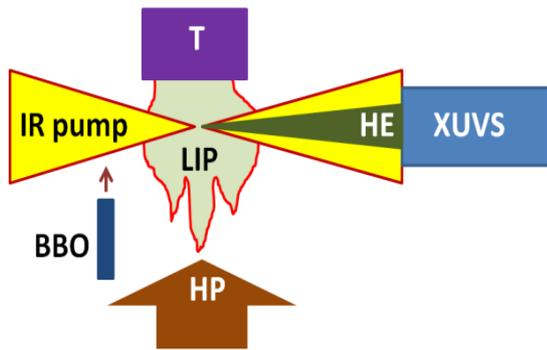
**Fig. 1.** Experimental setup for HHG in LIPs. IR pump: infrared (either 806 nm or tuneable NIR) driving femtosecond pulses; BBO: nonlinear crystal for second harmonic generation; T: solid target; HE: harmonic emission; XUVS: extreme ultraviolet spectrometer
