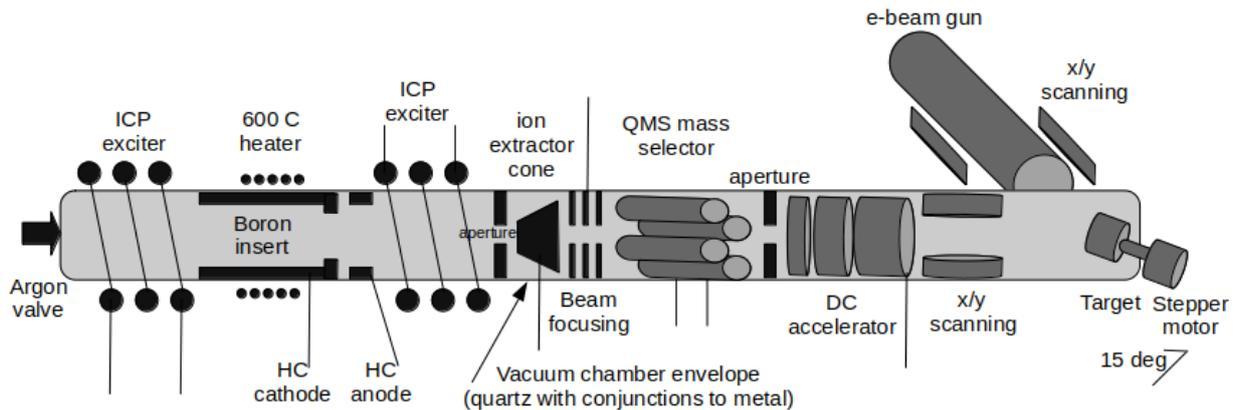
**Fig 1.** The boosted combined ICP-HC-ICP ion source in the full proposed implanter concept
