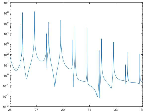
**Fig. 1.** Spectrum emitted by an atom driven by a laser field when the Planck constant is dependent upon the coordinates. It is evident a small redshift of the odd order harmonics. The redshift can be measurable.
