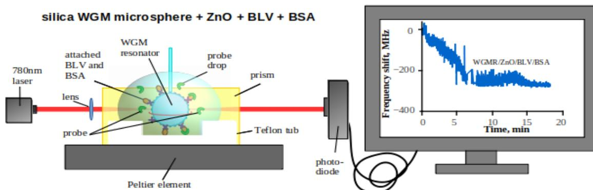
**Fig. 1.** Responses of cattle virus sensor based on antigen/antibody reaction modified silica microsphere WGM resonator
