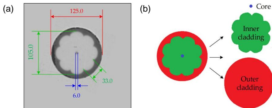
**Fig. 1.** (a) Microscope image of the EYDF cross-section with its geometrical measures, and (b) RGB representation of its outer cladding (red), inner cladding (green), and core (blue) used for the overlap factor estimation
