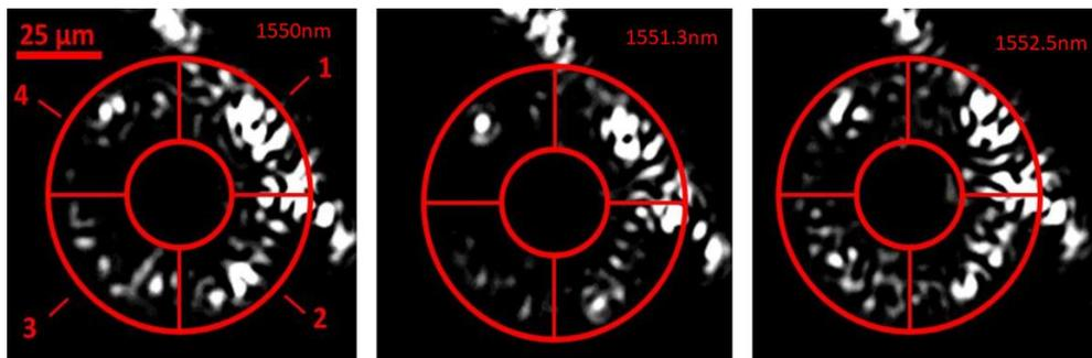
**Fig. 1.** 45µm PMMA WGM micro resonator attached to tapered fiber waist region, intensity using "Xenics Xs-5049" camera, for different wavelengths (1550nm, 1551.3nm and 1552.5nm)
