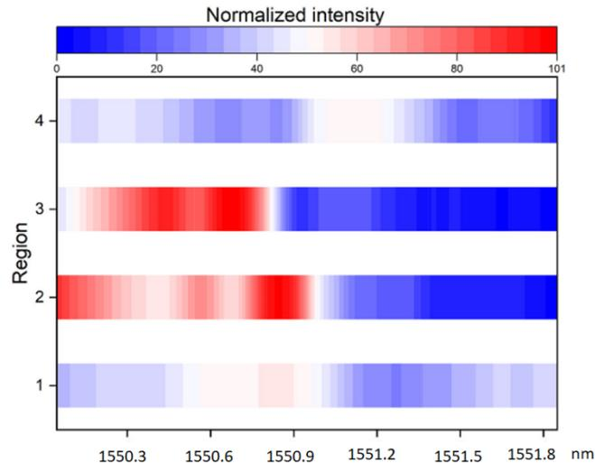
**Fig. 1.** Normalized intensity map based on wavelength changes for 50µm PMMA WGM micro resonator
