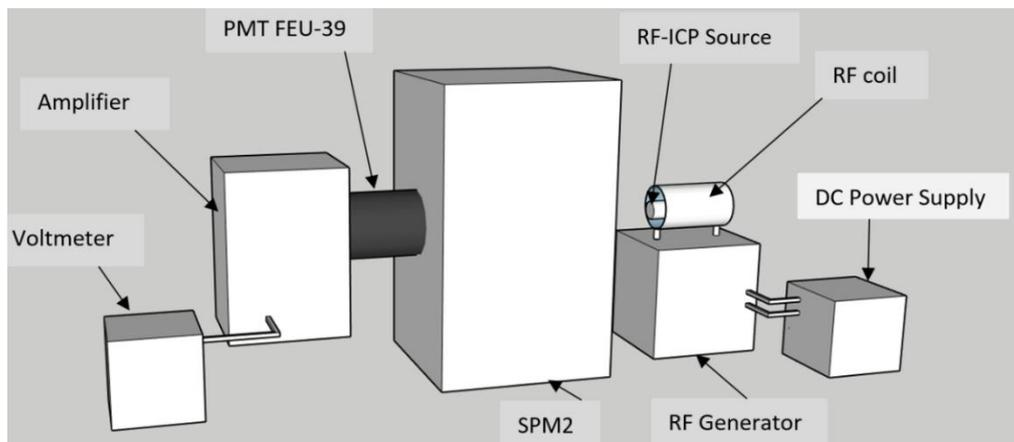
**Fig. 1.** Schematic of the experimental sett-up for branching fraction measurements
