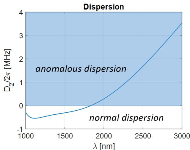
**Fig. 1.** Dispersion for  $R=332 \mu\text{m}$  belt type WGMR
