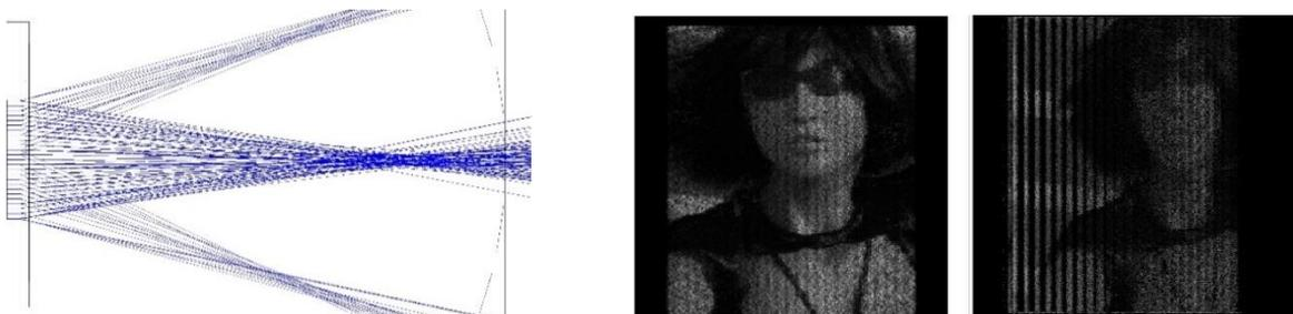
**Fig. 2.** Image simulation for 0° and 25° (1/2 of image, black lines are space multiplexion phase)
