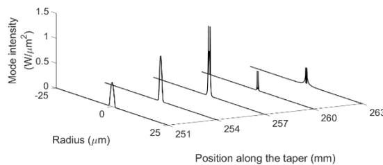
**Fig. 1.** Normalized Mode intensity profile along the tapered fibre
