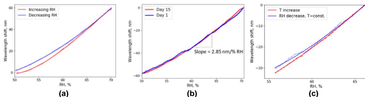
**Fig. 2.** Experimental results: **(a)** hysteresis; **(b)** repeatability, stability, sensitivity; **(c)** temperature dependence
