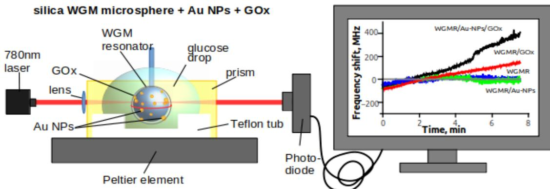
**Fig. 1.** Responses of glucose sensor based on differently modified silica microsphere WGM resonators: bare resonators - WGMR (blue curve), resonators coated with gold nanoparticles - WGMR/Au-NPs- (green curve), resonators coated with glucose oxidase layer – WGMR/GOx (red curve) and both layers to enhance sensitivity and provide selectivity - WGMR/Au-NPs/GOx (black curve)
