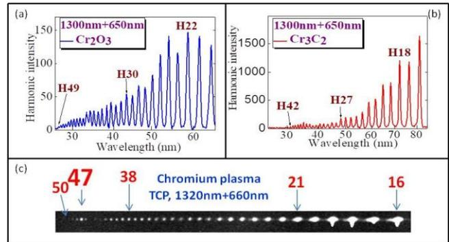
**Fig. 2.** Harmonic spectra from  $\text{Cr}_2\text{O}_3$ ,  $\text{Cr}_3\text{C}_2$  and Cr plasmas using tuneable NIR driving pulses. (a) HHG in  $\text{Cr}_2\text{O}_3$  LIP using 1300 nm + 650 nm driving pulses. (b) HHG in  $\text{Cr}_3\text{C}_2$  plasma using 1300 nm + 650 nm driving pulses. (c) HHG in Cr plasma using 1320 nm + 660 nm driving pulses at best conditions of plasma formation
