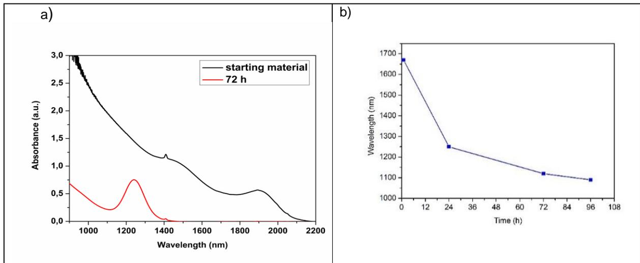
**Fig. 1.** Aging of QD PbS by storage of solution CQDs in the presence of oleylamine-oleic acid mixture: a) absorption spectra of samples; b) Dependence of the absorption spectra from the storage time
