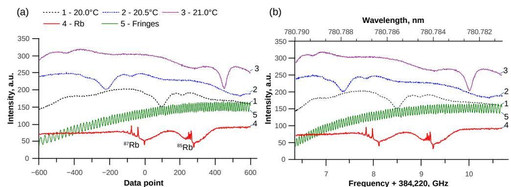
**Figure 2.** The temperature scanned WGMR resonance spectra for three different temperatures and two reference signals. (a) Before calibration, the laser scanning was obviously nonlinear, since at the beginning of the triangle signal the laser frequency scan was slower. (b) After calibration using both references for an almost linear absolute frequency scale.
